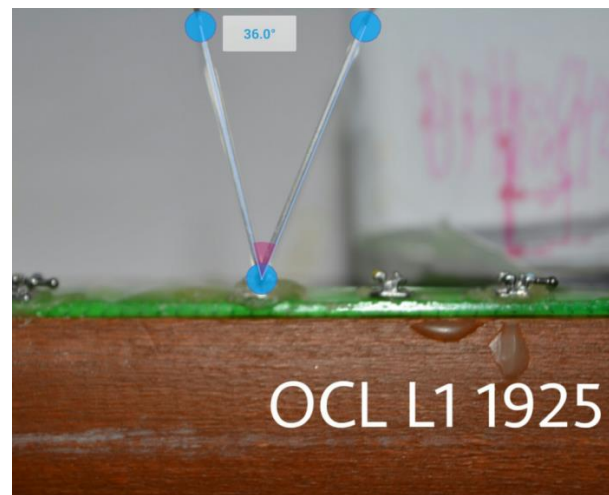
Figure 2: measuring angles with Protactor
